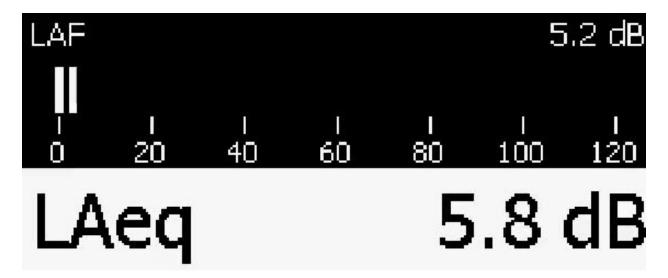
The noise measurements are conducted with Class 1 Bruel & Kjaer sound analyzers (2270 G4 and 2250-L G), equipped with type 4955-A low-noise and free-field microphones, which can measure down to 5 dB(A) (we also have type 4189 microphones that features a 16.6-140 dBA-weighted dynamic range). The sound analyzers are installed into a hemi-anechoic chamber with a close to 6 dB(A) noise floor. A Bruel & Kjaer Type 4231 is used before every noise measurement to calibrate the sound analyzers.
